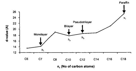
Fig 6. Representative XRD diagram of the fine clay smectite of Vertisols treated with alkyl ammonium chlorides (Source : Ray *et al.*, 2003)
