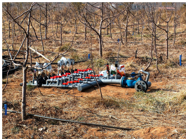
The control head of the fertigation system used in the experiment. Each treatment was operated through a separate water and nutrient supply. Photo by IPI.
