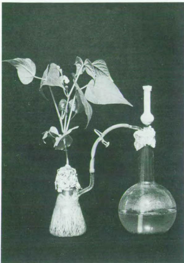
Fig. 2 Axenic nutrient solution culture of bush beans. The flask is connected with a water reservoir. ( Trolldenier [1972a] )
