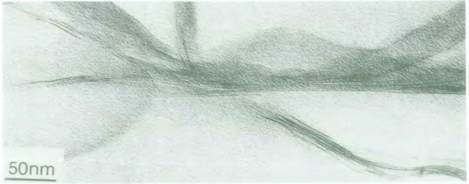
Fig. 14. Characteristic particles of a Na smectite (Hectorite) 10^{-3} M NaCl. – 0.032 bar – TEM (photo: Tessier)
