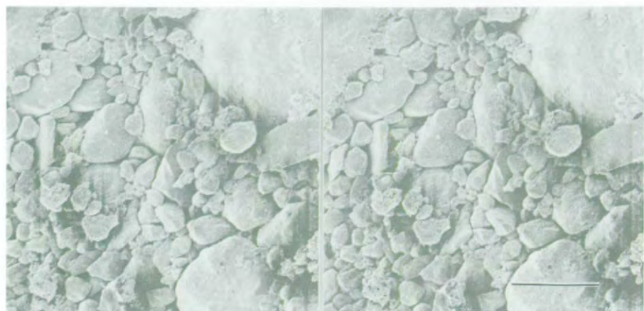
Fig. 2. Stereo pair of compacted area of naked grains on soil surface after being submitted to rain simulation with distilled water (bar 100 \mu\text{m} ).
