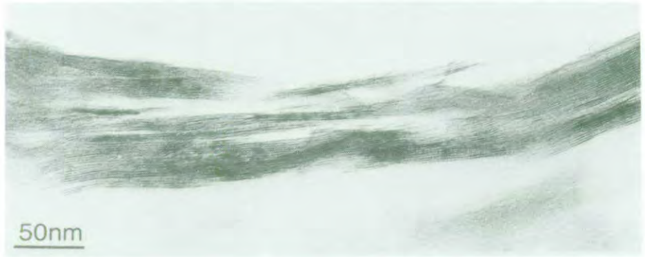
Fig. 15. Characteristic particle of a Ca smectite (Greek) 10^{-3} M \text{CaCl}_2 – 0.032 bar – TEM (photo: Tessier)
