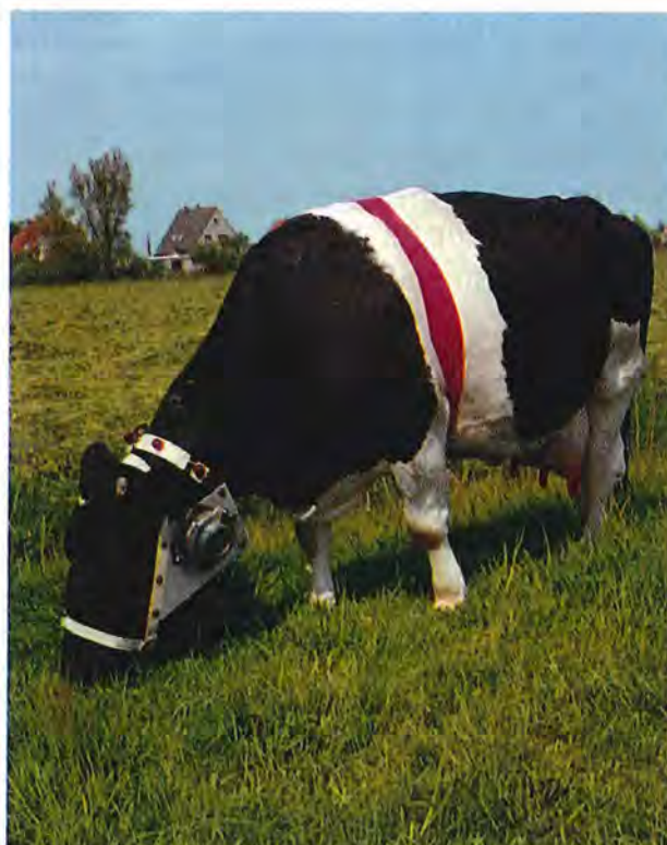
Cow with a vibracorder, an instrument to measure grazing frequency and duration in pasture experiments
