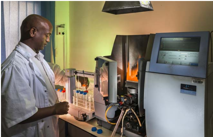
Photo 1. Measuring Ca, Mg and Na from soil extract by AAS (Atomic Arbitration Spectroscopy). Photo by E. Sokolowski.
